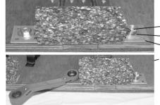
Place the flat bars directly on the wood (1), insert the washers (2), and finally the nuts (3)
